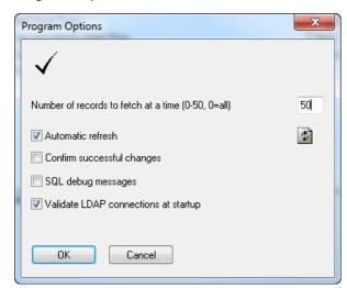
Number of records to fetch at a time (0-50, 0=all) []: Netop Security Manager fetches Security Database records to the Records Pane in batches. Specify in the field a number in the range (default: 50).
