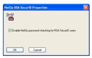
☑ Enable Netop password checking for RSA SecurID users: Leave this box checked to request a Netop password in addition to the RSA SecurID user name and PASSCODE from a connecting Guest to apply triple-factor security (default: checked).
