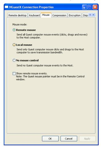
Use the *Mouse* tab to select mouse mode, i.e. which mouse events should be sent to the Host computer. Sending fewer mouse events saves transmission bandwidth.
