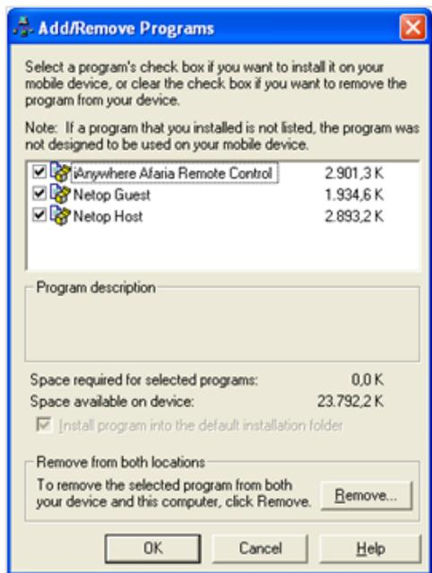
The **Add/Remove Programs** window will display all programs that you can install on the mobile device from the desktop computer. If a check box has been selected, ActiveSync has detected that the program has been installed on the mobile device.
